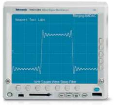
than 6 volts, as per the tabulated results. Newport Test Labs measured signal-to-noise ratio at 116dB unweighted and 122dB Aweighted using 16-bit/44.1kHz, with the Aweighted figure improving to 126dB when tested at a 24-bit/48kHz sample rate.
